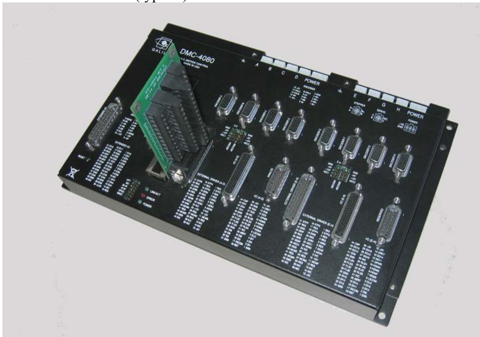
Figure 2: ICS installed on DMC-4000
