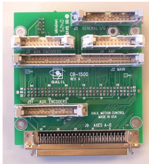
CB-1500 Interconnect Converter Board (CB-1500-96-100 shown)
