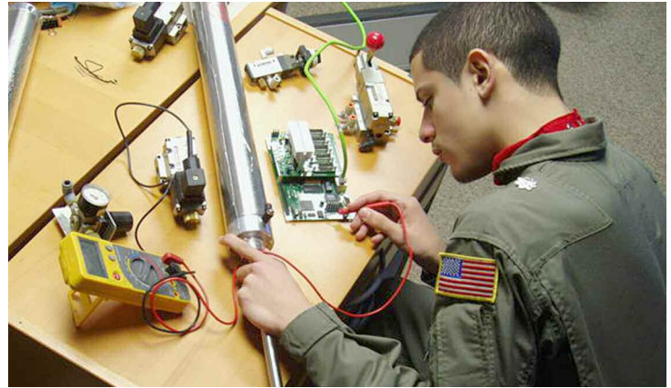
Galil's controller is used by the Project Kitty Hawk team to control the pitch, roll and yaw of their flight simulator.
