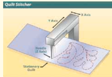
(Figure 2) Once the Quilt Stitcher Visual Basic application is launched, the user chooses a stitch pattern, represented by a two dimensional image on the right.
