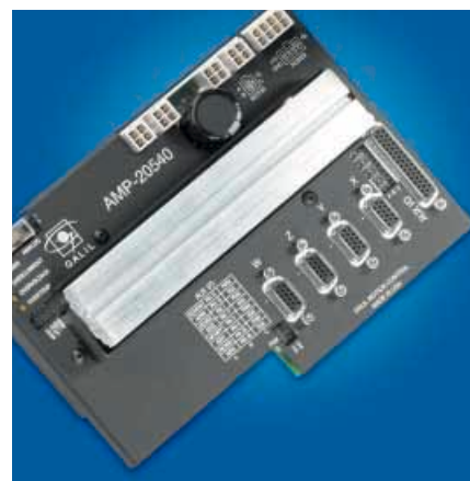
Galil's DMC-21X3 controller with sandwiched amplifiers is designed for Ethernet applications.
