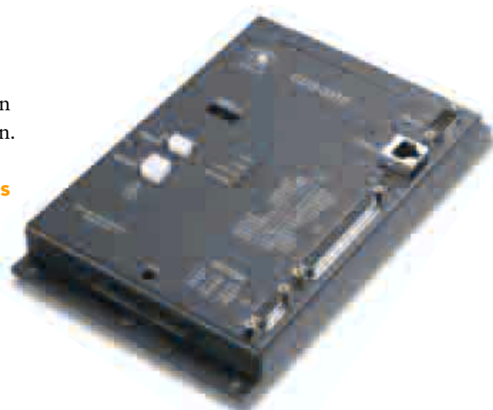
The new Galil CDS-3310 is an example of an Ethernet based single axis controller and amplifier that can be used in a fully distributed control system.
