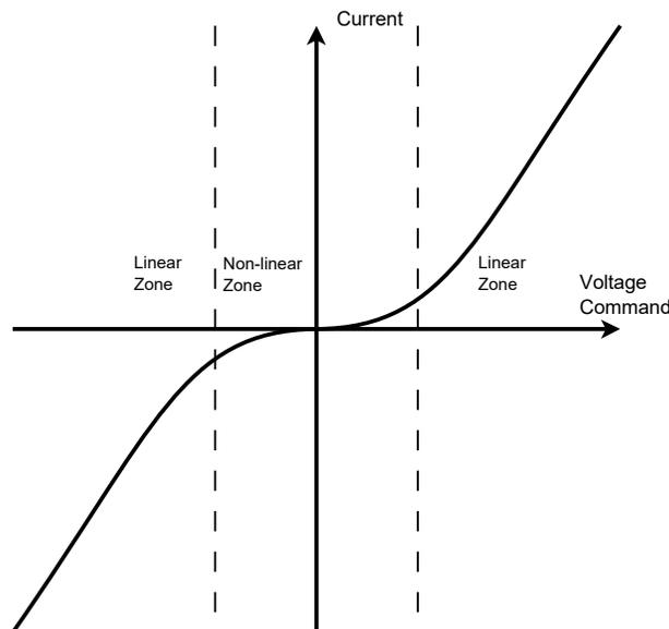
*Figure 2: Output of Voltage Amplifier in Chopper Mode*
